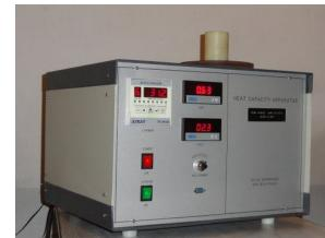
This apparatus is designed to measure Heat Capacity of nanofluids from RT+5°C to 70°C.
