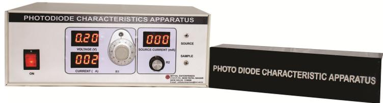
A **photodiode** is a type of photodetector capable of converting light into either current or voltage, depending upon the mode of operation. Photodiodes are similar to regular semiconductor diodes except that they may be either exposed or packaged with a window. Many diodes designed for use specifically as a photodiode will also use a PIN junction rather than the typical PN junction.
